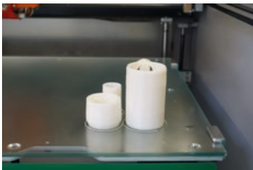
Additively manufactured components for the ventilator with the HAGE3D 3D printer.
