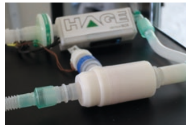
A 3D-printed valve controls the pressure supply of the oxygen.
